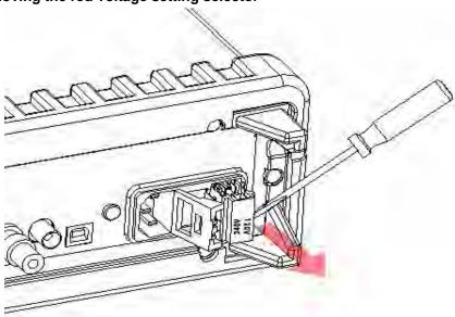
Step 4: Remove the damaged power line fuse
