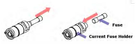
Step 5: Reinsert and secure the current input terminal fuse holder
