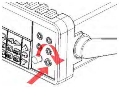
Step 3: Remove the current input terminal fuse holder
