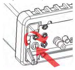
WARNING Before reconnecting the power line cord to your multimeter, ensure that the power switch is in the "POWER OFF" position.
