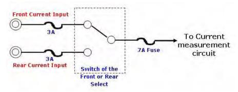
The two main fuses located in the front and rear current input terminals of your Model 2100 are 3A, 250V, 5x20mm fast-acting glass fuses (Keithley Instruments part number FU-99-1). The additional current input fuse is a 7A, 250V, 5x20mm fast-acting ceramic tube fuse. See the following text for instructions on how to replace these fuses if they become damaged.
