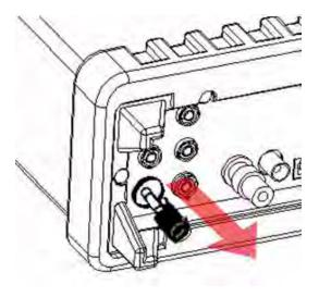
Step 4: Remove and replace the damaged fuse
