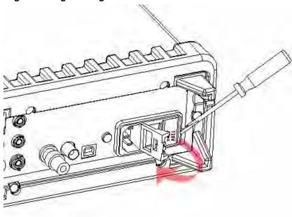
Step 3: Remove the red voltage setting selector
