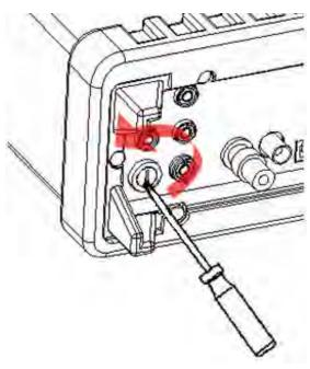
Step 3: Remove the current input terminal fuse holder
