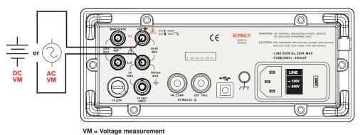
**NOTE** Follow the same procedure when using either the front or rear panel terminals (refer to Figure 3-3).
