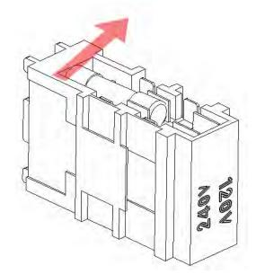
Step 5: Replace the power line fuse
