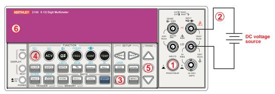
Input resistance = 10M $\Omega$  on 1000V and 100V ranges: > 10G $\Omega$  on 10V, 1V, and 100mV ranges.
