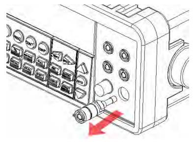
Step 4: Remove and replace the damaged fuse
