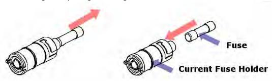
Step 5: Reinsert and secure the 7A current input terminal fuse holder
