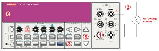
Input Impedence = 1M  $\Omega$  in parallel with < 100pF (Warning: Maximum input = 750V RMS, 1000V peak, 8x10' V-Hz)
