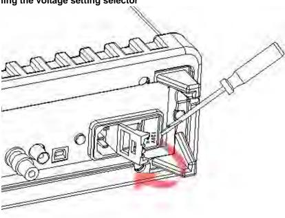
Step 3: Remove the red voltage setting selector
